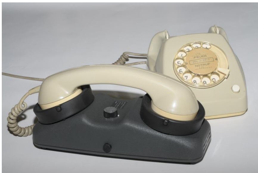
Figure 2 An acoustic coupler that converts electric signals to and from sounds.
